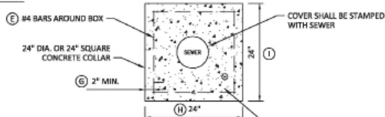
WW - FIGURE 04: VALVE & VALVE BOX DETAIL
