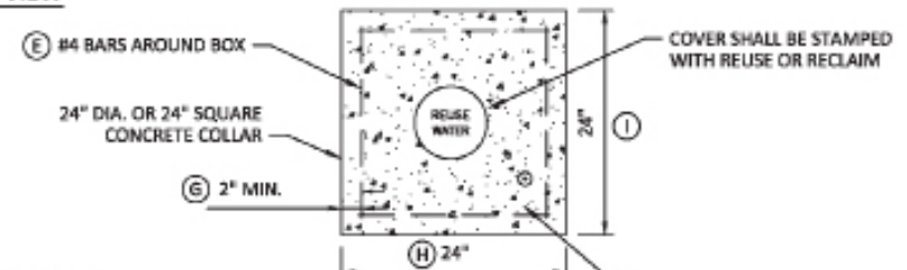
RW - FIGURE 04: VALVE & VALVE BOX DETAIL
