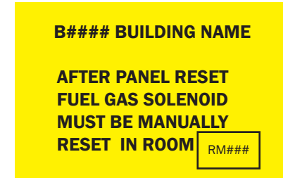
FIGURE 28-02 GAS SOLENOID PLACARD
